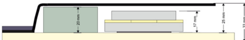
Build-in depth of a Re:sound I U mini Board
