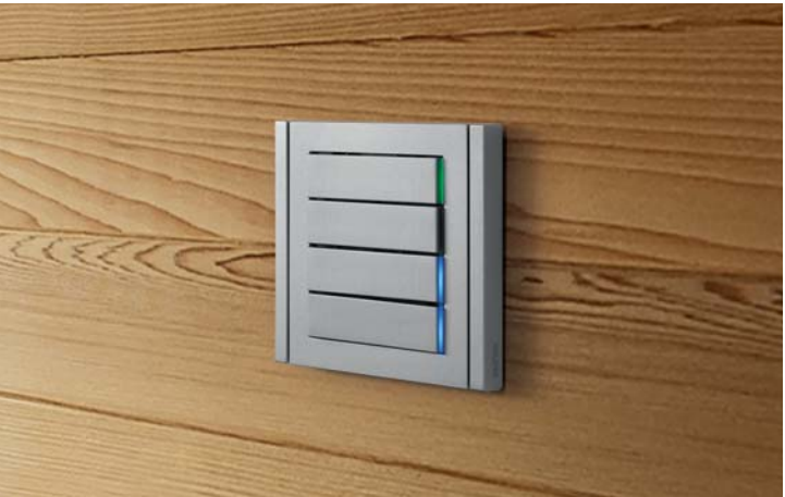
E12 - 4 rectangular rockers. Finishing metallized plastic, color silver, blu/green LED. Dimensions: mm 94 x 86 x 8
