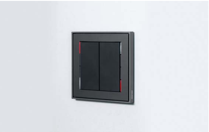
E12 - 2 rectangular vertical rockers. Rockers finishing plastic, color black; frame and plate finishing brushed metal, color titanium, red/white LED. Dimensions: mm 86 x 86 x 8
